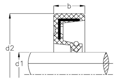
$\begin{array}{ll} b & = 8 \\ d1 & = 45 \\ d2 & = 60 \\ Material = NBR \end{array}$
